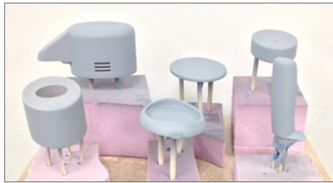
Individual components were sanded, primed, and painted. Buttons and emblems were 3D plaster printed.
